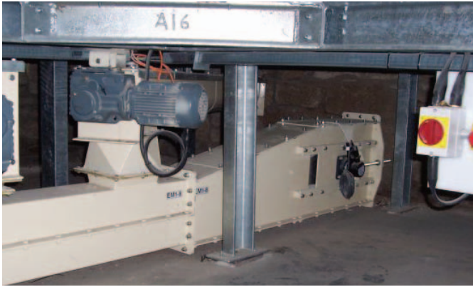
Conveying malt from storage bins to the grist mill.
