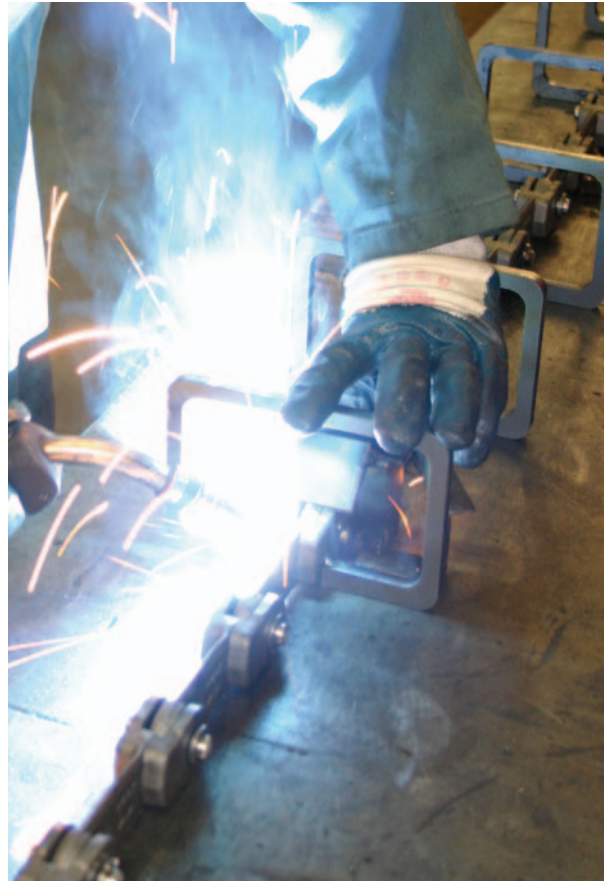
The chain and flight configuration is designed and fabricated to suit the application.
