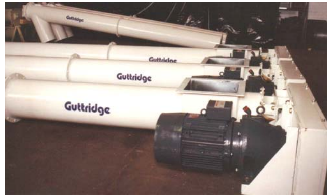
Tubular Screw Conveyors feature heavy duty casings as standard.
